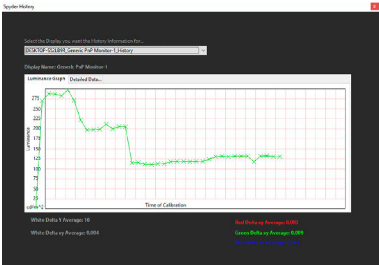
Example of several measurements. The decrease in luminance over time is clearly visible here.
